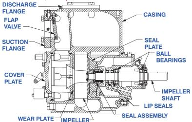
**Shown with Optional Suction & Discharge** Spool Flanges (Available in ASA or DIN Standard Sizes).
